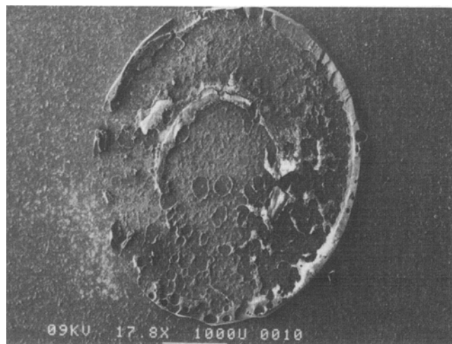
Fig. 15 SEM micrograph of an adherence-tested sample coated with a 5 \mu\text{m} DLHC
